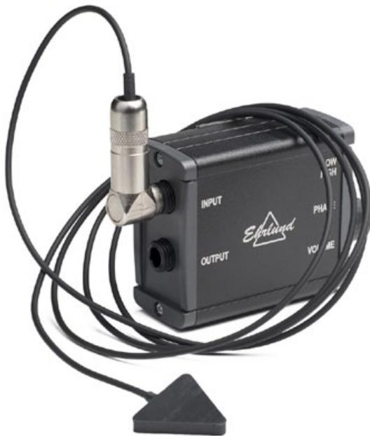
*The pickup is connected to the preamp at the INPUT jack socket. The mixer/amplifier is connected to the OUTPUT jack socket. Note that the preamp automatically switches on when a connection is made in the OUTPUT jack socket.*
