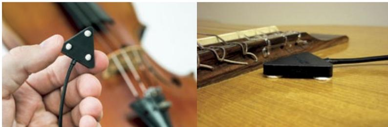
*The adhesive needs to be shaped into small balls about 3-4 mm in diameter and attached to the corners of the pickup. Important: Never attach adhesive to the middle of the pickup.*
