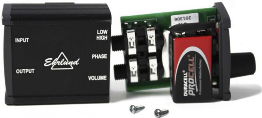
4. The Preamp will open on the volume control side. Carefully pull away the cover until you reach the battery. You can now replace the battery.
